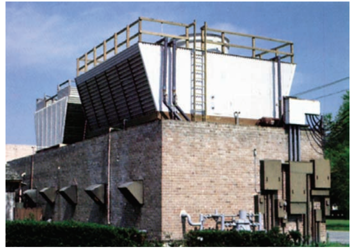
Marley Series 10/Series 15 Cooling Tower —Splash-fill design for use at high temperature or where poor water quality prevents the use of film fill. Wood structure available in treated Douglas Fir or redwood. Tower cells available from 50 to 1,090 m 3 /hr.
